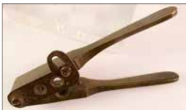
Lot # 2420 Rare Civilian Brass .44 Colt Double Bullet Mold 1850-1870 . Rare brass civilian double cavity .44 caliber bullet mold for conical and ball. Brass bullet mold with steel sprue cutter, typical of civilian market and generally used for Colt's .44 caliber Dragoon and Army
